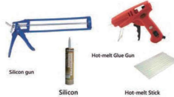
Prepare the tools and materials as pictures. Apply the silicon on 4 corners and middle on the back of panel. Then, apply the Hot-melt glue on 4 corners.
